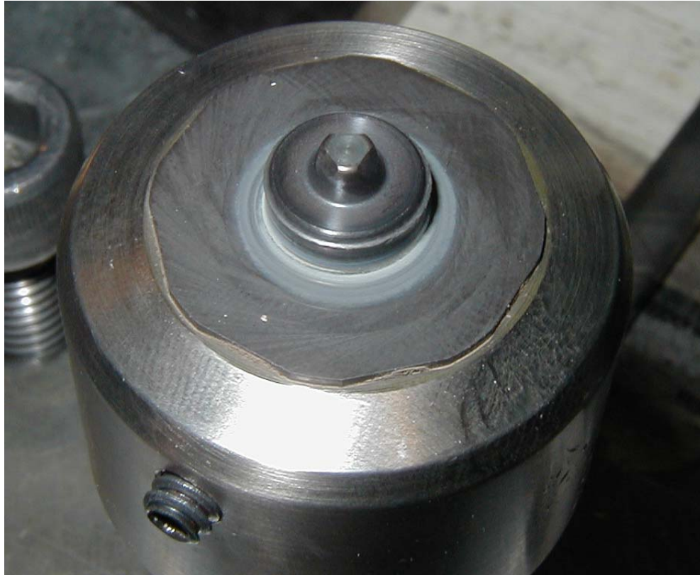
FSSW tool made of polycrystalline cubic boron nitride (PCBN)
