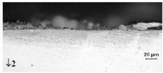
Figure 6. Fracture appearance (A) after shear-tensile testing and cross-section (B) of a FSSW-joint in 1.5 mm Dogal 600 DP. The numbered arrows (↓1 to ↓4) indicate the position of the micrographs.
